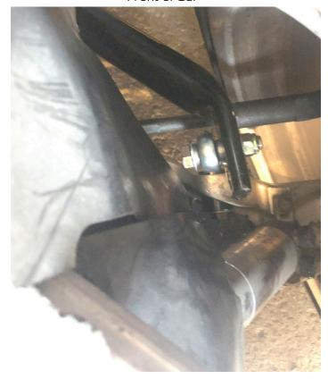
Endlink is on the front of the control arm and on the inside of the sway bar.
